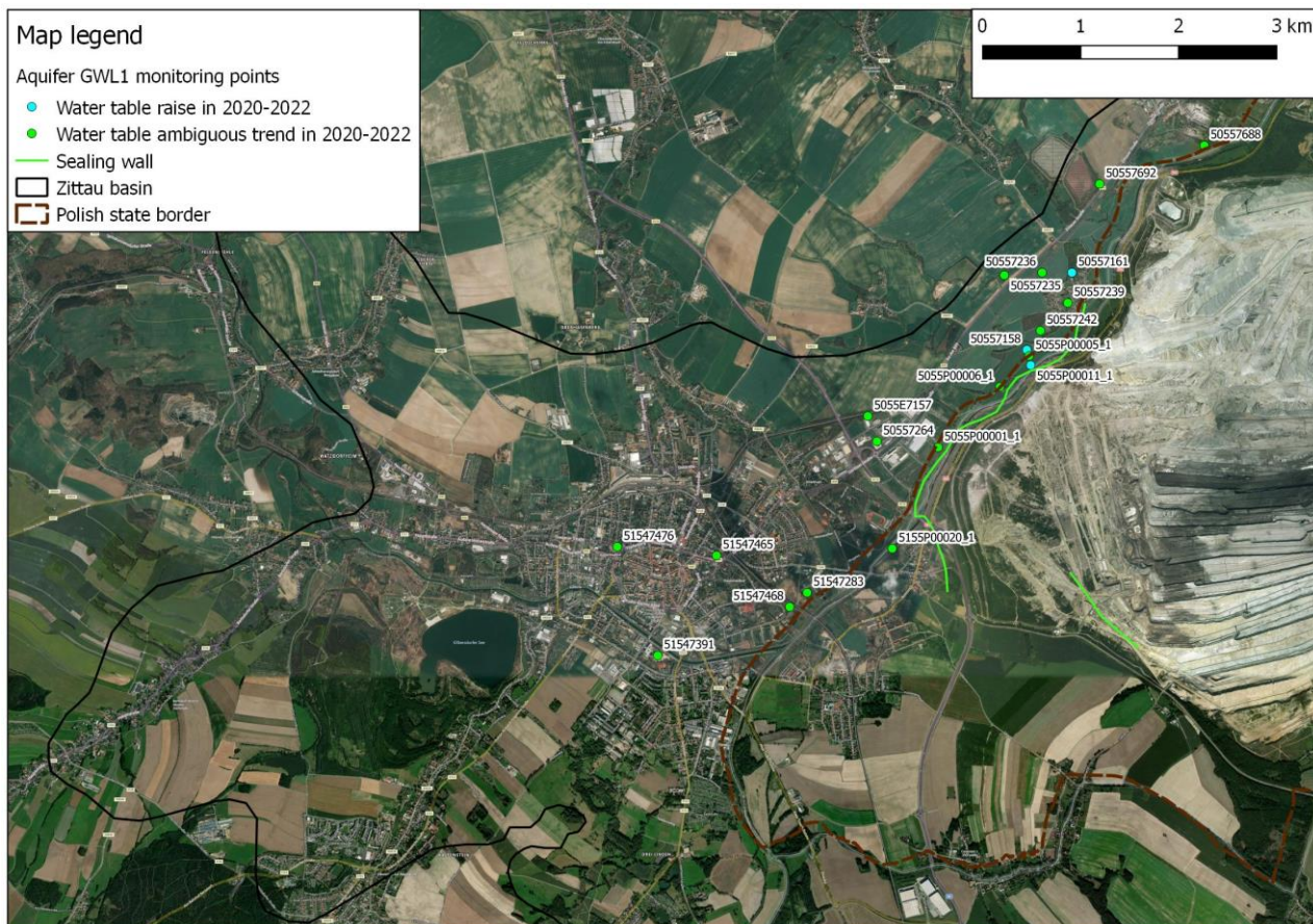
Fig. 3. Location of the groundwater wells monitoring the GWL 1 aquifer.
