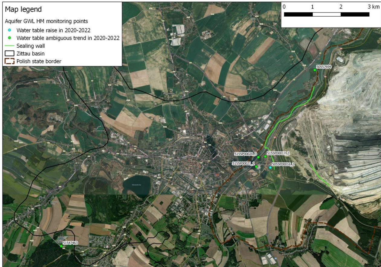
Fig. 14. Location of the groundwater wells monitoring the GWL HM aquifer.
