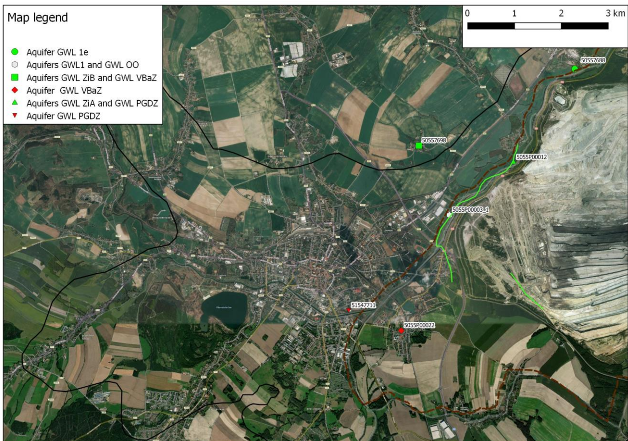
Fig. 28. Location of the groundwater wells monitoring the aquifers: GWL 1e, GWL1 and OO, GWL ZiB and VBaZ, GWL VBaZ, GWL ZiA and PGDZ, GWL PGDZ.
