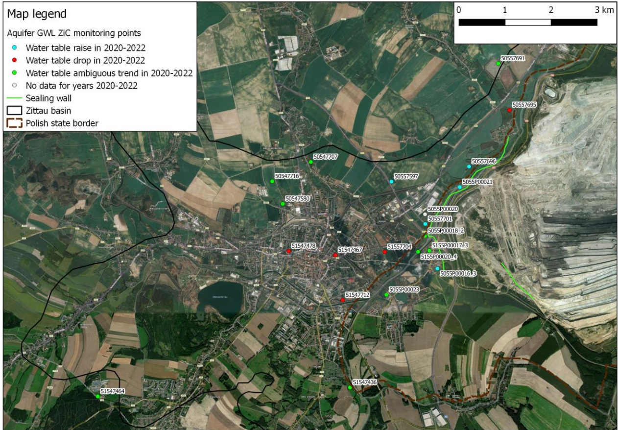
Fig. 20. Location of the groundwater wells monitoring the GWL ZiC aquifer.
